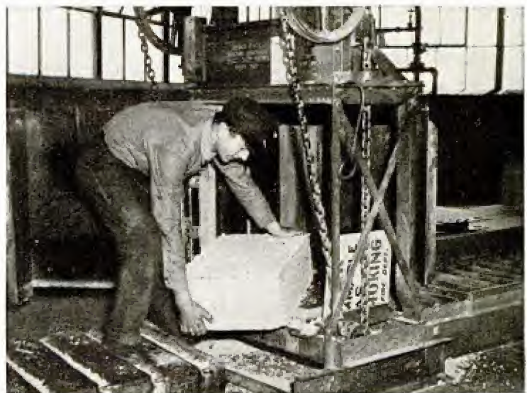
Check and double check—this huge rubber pontoon float made for the U. S. Army must be flawless for its future role under hail of shells Workmen removing a "cake" of Chemigum, synthetic developed by the Goodyear Co., from a press. Cakes are converted into war materials
